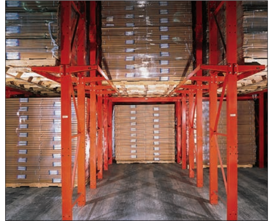
MECO OMAHA Drive-in Rack installation. Custom-designed for high density storage and efficient handling.
